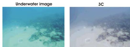
Figure 4. Example of 3C color compensation algorithm for underwater scenes
