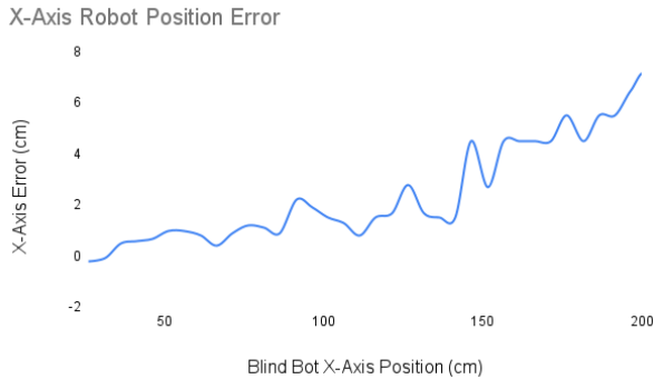
Fig. 5. Position error of AprilTag based robot detection system along the x-axis of the Blind bot
